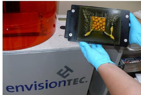
Once the print job is complete it's raised out of the liquid base plate and ready for cleaning.
