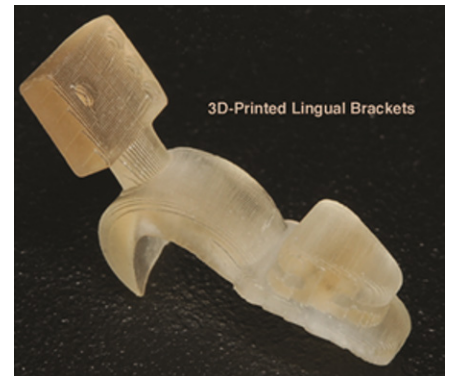
An example of a 3D-Printed Lingual Bracket
