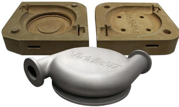
Casts can be directly printed on the Viridis3D RAM system.
