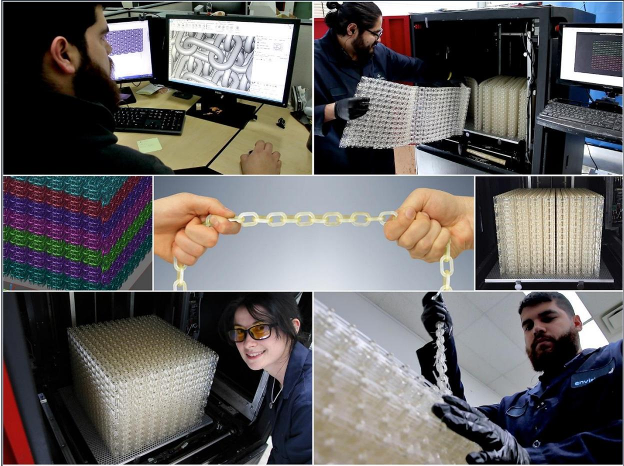
*The EnvisionTEC Mega-Chain is a 328-foot chain that was 3D printed in a durable new material, E-RigidForm. Designed by EnvisionTEC 3D Builder Robert Montes (upper left and lower right), the chain features 6,144 links, each measuring 1.5 inches. The print job was processed with support from colleagues Erica Finkowski (lower left), Josue Nunes (upper right) and Jason Spurlock (not shown).*
