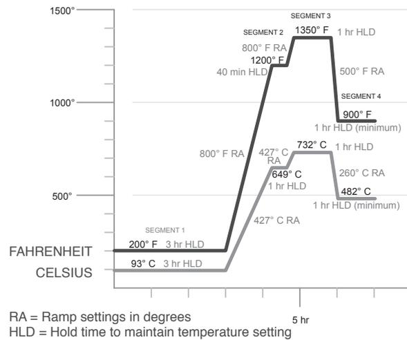
To help prevent porosity, slow down the initial ramp time for EnvisionTEC materials. The critical range is between 1-500 degrees F.
