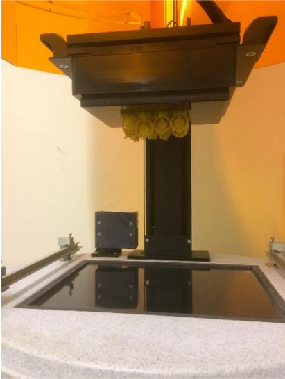
Items printed on Rapid Model's Perfactory 3D printer.
