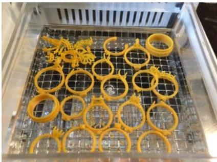
Rings produced on the Perfactory 3D printer. [Link](#)
