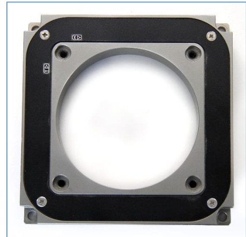
This is photograph of the EnvisionTEC Enhanced Resolution Module, which moves a half pixel in X and Y, to slightly shift the second exposure in its DLP machines and reduce stairstepping in a sophisticated 3D anti-aliasing technique. The projector shines through the center of the module.
