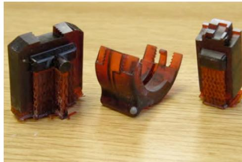
Trevor continued: "We used the Perfactory® to build the precision parts from which we could then build a rapid tool to create test parts in the exact production material before committing to the expense of the production tool. This was a key part of the development process and allowed us to achieve the optimum design."
