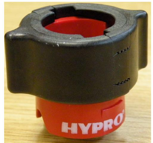
The Guardian AIR Twin is a crop spraying nozzle design, which incorporates a new attachment concept. The patented attachment method is a twist ring that eliminates the traditional attachment method requiring separate caps. This precision part required the tightest possible tolerances and the capabilities of the Perfactory® successfully met these requirements.
